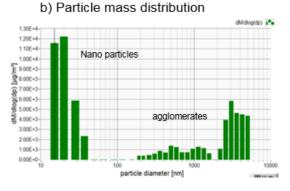
Figure 2: Measurements at workplaces with soldering a) total particle number concentration, b) particle mass distribution
